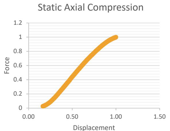
Figure 3 - Normalized Force/Displacement curve for an implant in Static Axial Compression.
