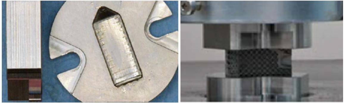
Figure 2 - Implant in mechanical testing with Implant test blocks (left) demonstrating recessed cavity for containing implant during test, and as loaded configuration (right) with an implant in the mechanical test stand between blocks.
